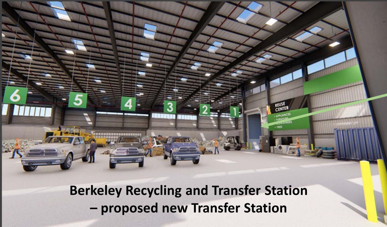
Loading dock integrated with tip floor to facilitate recovery of reusables, bulky items, and universal waste
