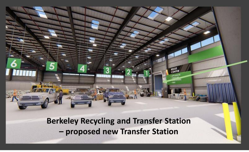
Loading dock integrated with tip floor to facilitate recovery of reusables, bulky items, and universal waste
